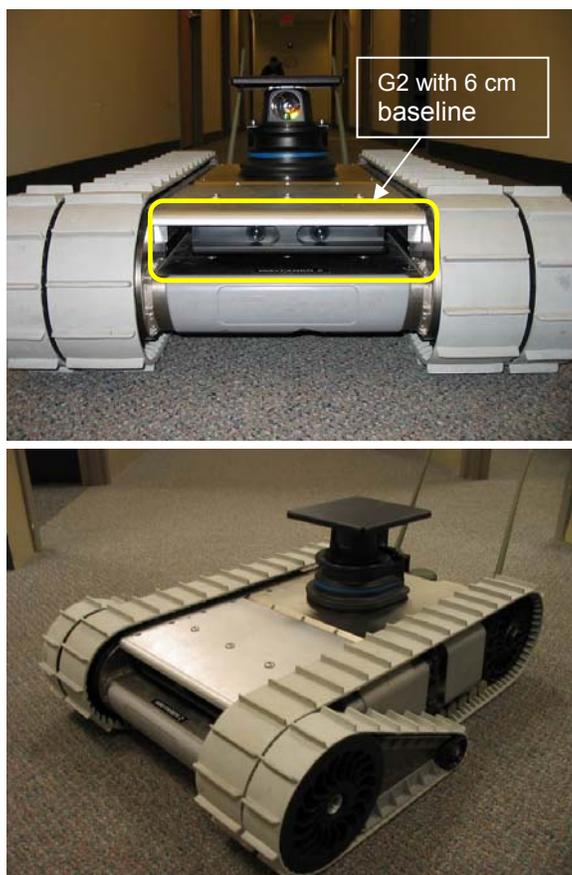
**Figure 5. iRobot Wayfarer: Autonomous robot navigation application.**
