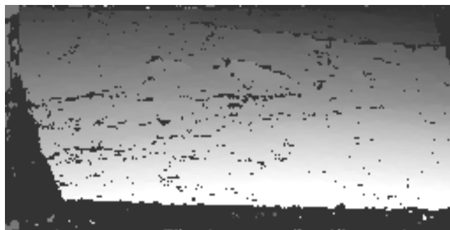
Figure 10: Temporally filtered stereo disparities for a pair of images from Figure 9.
